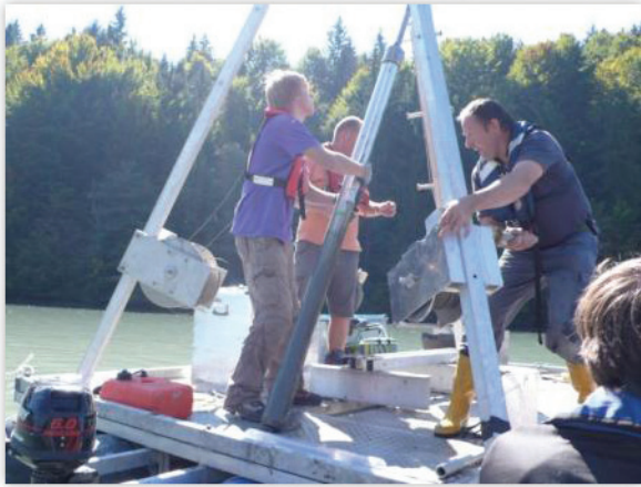
Removal of sediment probes for underground investigation in the reservoir Feistritz/Ludmannsdorf (Drava)
